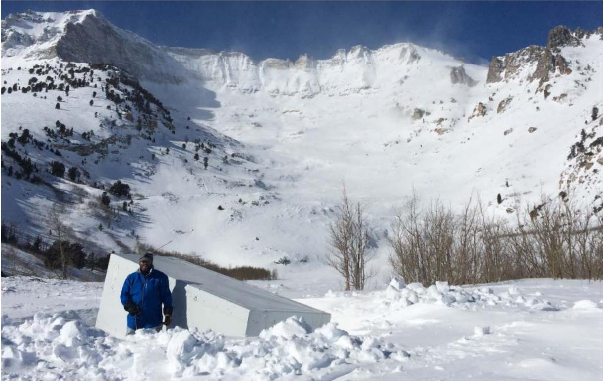
Photo 2: Damaged observed at Hole in Mountain SNOTEL after avalanche. The SNOTEL shelter, which houses the site's electronics, was swept 200 feet downhill of its foundation. Photo taken January 2016.
