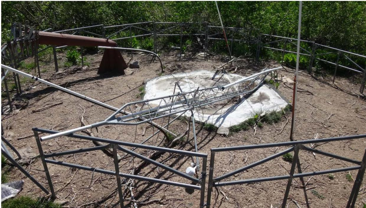
Photo 3: Damaged observed at Hole in Mountain SNOTEL after melt-out. The avalanche bent over the brown precipitation gage and instrument tower. The snow pillow which weighs the snowpack is the white object under the tower. Photo taken June 2016.
