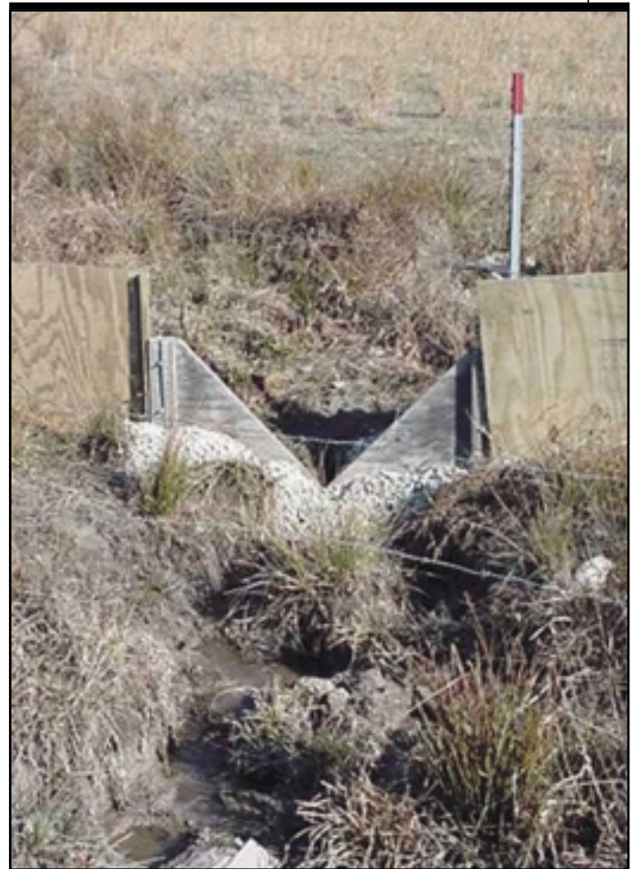
A V-notch weir to measure water flow.
