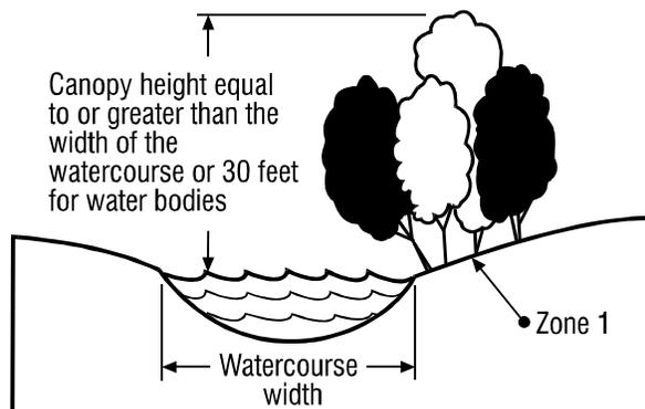
Figure 5. Canopy height for water temperature control.
